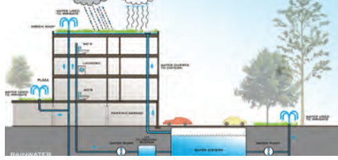
Rain Water Harvesting
